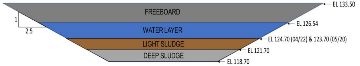
FIGURE 15 ELEVATION DRAWING OF THE EXISTING LAGOON SYSTEM
