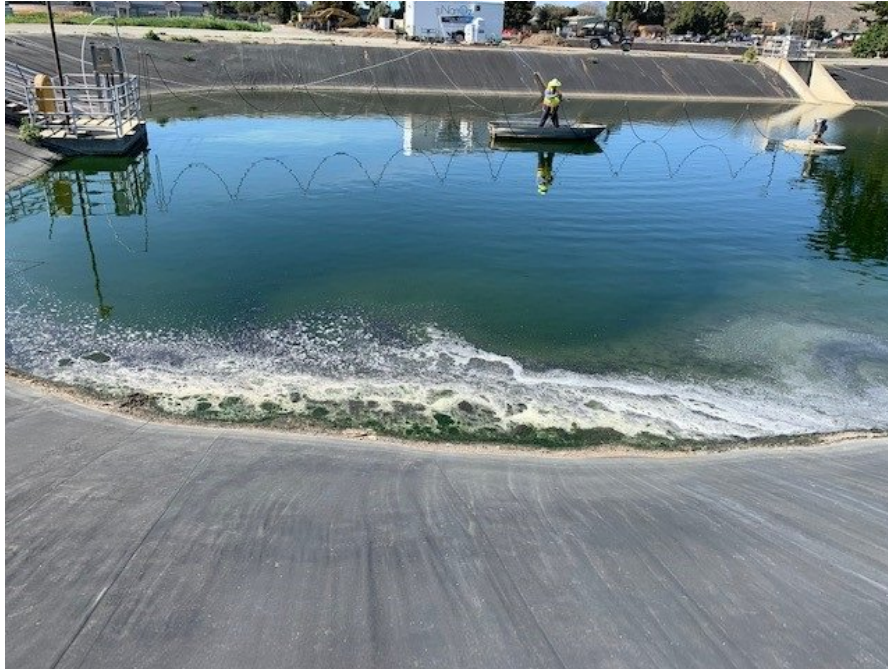
FIGURE 20 STAFF OBTAINING GRAB SAMPLE OF SLUDGE
