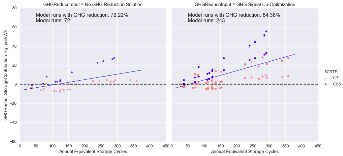
Figure 33: GHG Reduction kg/kWh vs Annual Cycles for Residential Storage with Solar on New Rates
